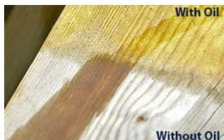
Water is absorbed into the wood without oil
