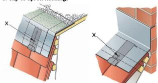
x = For moderate to severe exposures additional fixings should be positioned at not more than 75mm from the free edge. Secure clips with Copper Nails.
