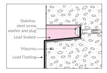
Wide joints over 18mm will require a more substantial fixing. Hall Clip Plus can be used for chase heights of 18-26mm. It is recommended that stainless steel screws and washers are used at 450mm centres on flashing lengths of no longer than 1500mm. The joint should be prepointed with mortar and then pointed with BLM Lead Pointing Sealant.
