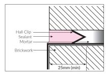
The joint should be at least 6mm wide to allow Hall Clips to be inserted to hold the Lead flashing in place before pointing in with BLM Lead Pointing Sealant.
