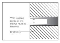
When removing mortar from an existing joint it is important to remove ALL the mortar to a depth of at least 25mm.
