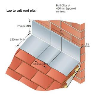
Edges clipped to suit exposure. Use Copper strip or Permastrip. No flashing piece to exceed 1.5m in length.
